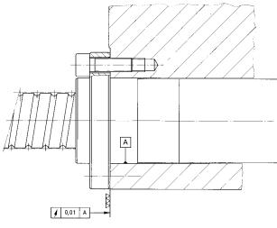
In order to ensure a proper function, we recommend the angularity of your flange locating surface to spindle axis be maintained, as indicated in the figure, i.e. also note alignment of bearing to guidance track.
