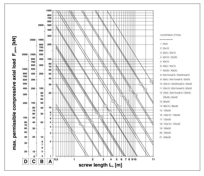
Steps for increasing the permissible compressive axial load
