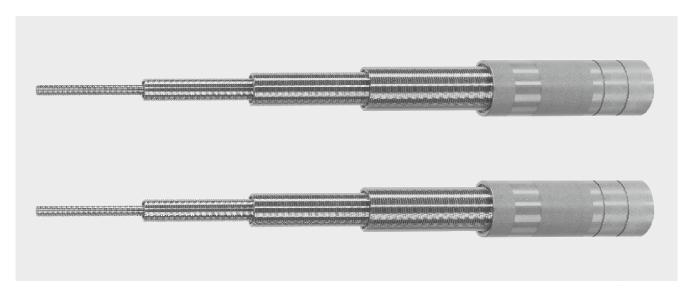
$\begin{array}{lll} \mbox{Telescopic Ball Screws} & = 4 \mbox{ stage} \\ \mbox{draw ratio i} & = 3.64 \\ \mbox{max. height } \mbox{h}_{\mbox{\tiny max}} & = 1,375 \mbox{ mm} \\ \mbox{largest } \mbox{$\varnothing$} & = 130 \mbox{ mm} \\ \mbox{dynamic load rate } \mbox{$C_{\rm dyn}$} & = 26 \mbox{ kN} \\ \mbox{max. number of rotation } \mbox{$n_{\rm max}$} & = 600 \mbox{ min}^{-1} \\ \end{array}$
